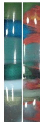
Fig.50. reduction of glass containing copper
