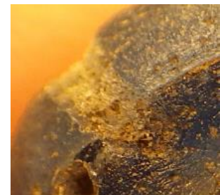
Fig. 40. Close-up of stringer scar in Bead 70 59.
